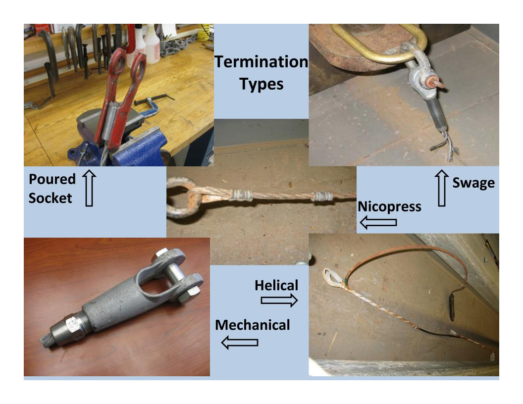
Poured-socket terminations and swaged fittings are principal terminations applied to break test samples that arrive unterminated
