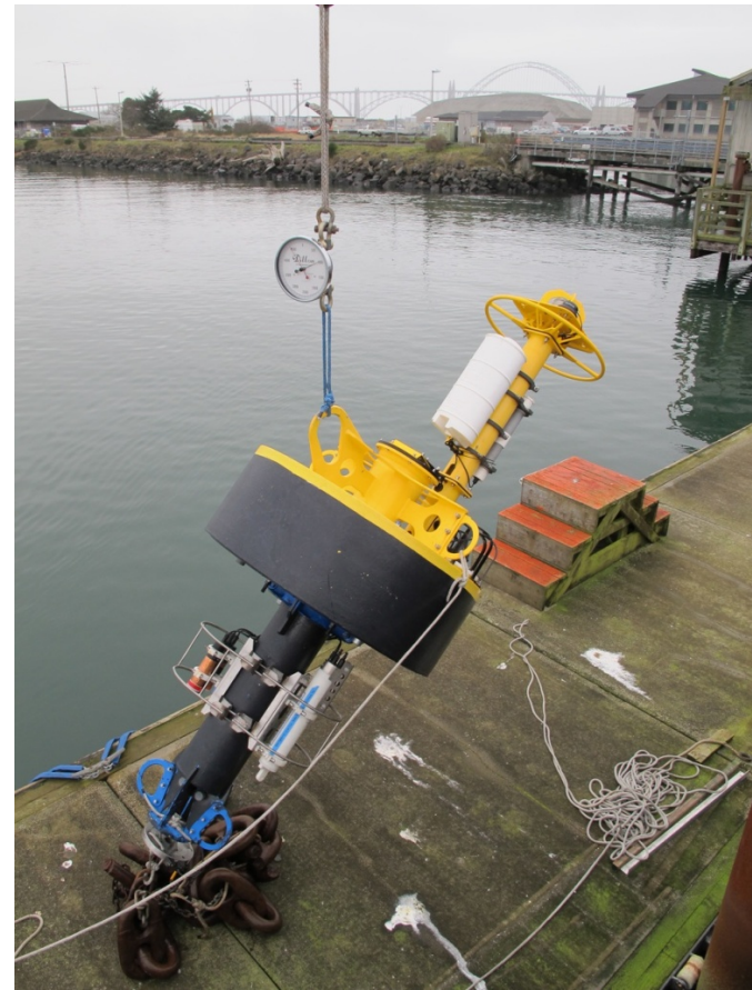
'Hardened 25 m surface buoy'
