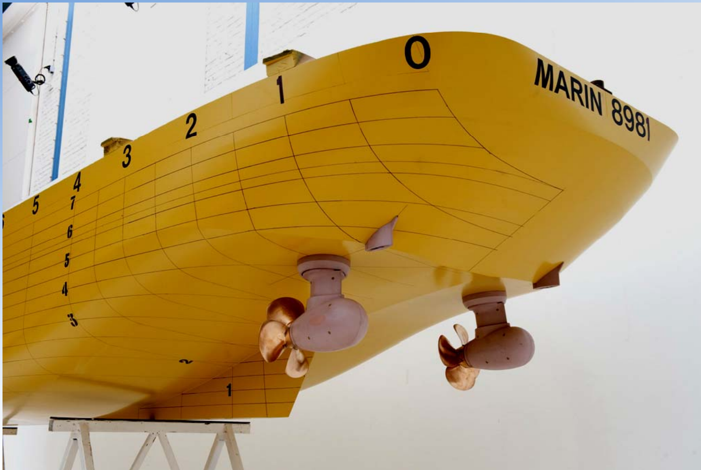
Stern view with tractor Z-drive units and ice stops
