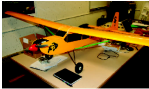
U. of Colorado UAV Laser Profing System installed in a UAS-capable Telemaster aircraft at C.U.
