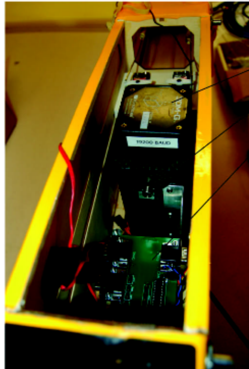
IMU laser altimeter electronics (payload computer, GPS, flash memory data storage)
