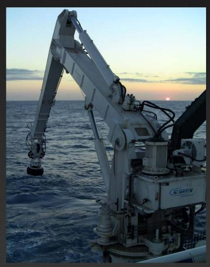
the system was designed to be able pass a four inch diameter fitting thru the docking head and crane sheaves to the winch level wind
