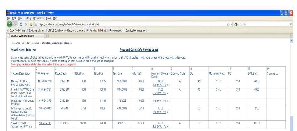
Each row in the form represents a particular winch system, wire rope or cable, and fairlead combination.
