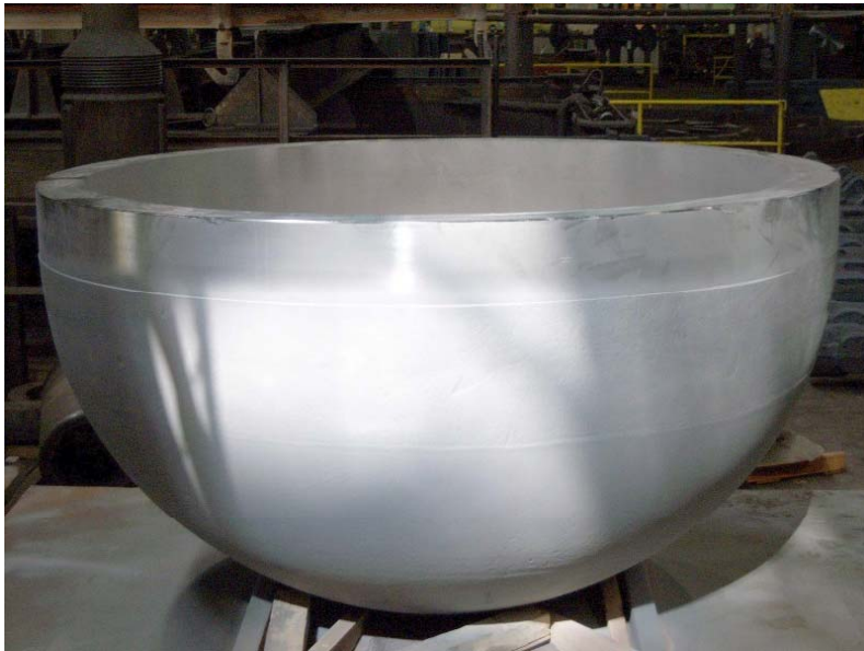
Final Forged Hemisphere with \approx 6 inch prolongation
