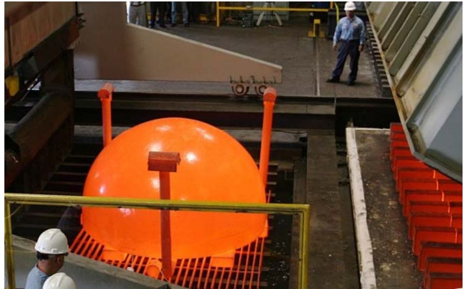
Hemisphere Heat Treatment and Water Quench
