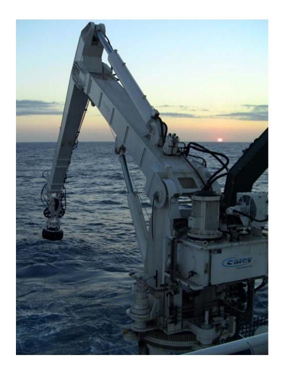
"Overall the entire system works very well. Launching and recovering utilizing the docking head reduces the number of personnel required from five to two (technician to run the crane & winch during deployment/recovery, one AB to take up tension on the cable while preparing to launch or after recovery, and to run the winch during long casts). The docking head stabilization feature reduces the wild pitching packages experienced previously, making operations safer for equipment and personnel."
