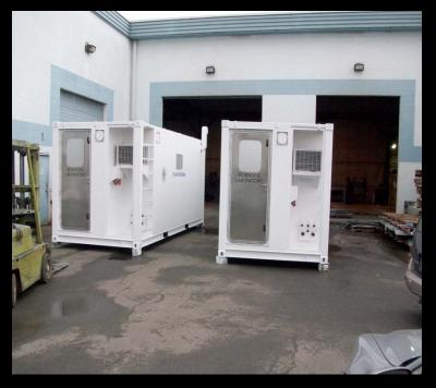
The two office of polar program's vans; Finished construction and ready for transport. One is an isotope van and the other a general purpose van.
