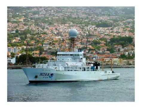
The second way, favored by the Cruise ship industry, is to install redundant antennas so that when one is blocked the other is not. Neither of these methods are particularly attractive for the UNOLS fleet but I believe each ship might be able to improve performance by judicious re-location of the existing antenna.
