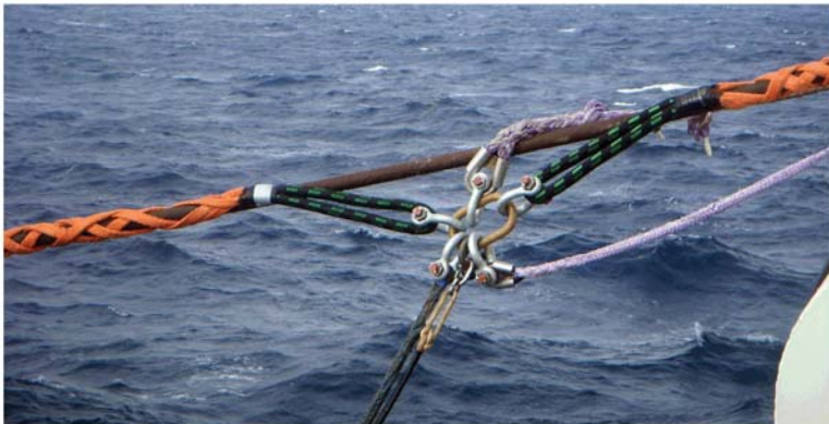
Cable separation rope rigging
