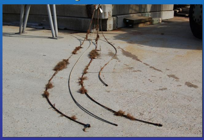
factory applied lube (left). Second was old rusty specimen unlubed and shows much growth and corrosion. Third was new and lubed with StanCore lubricant and CoreLube lubricator. This shows no fouling and little corrosion. The forth was an old rusty specimen that was lubed with StranCore. Shows some fouling.
