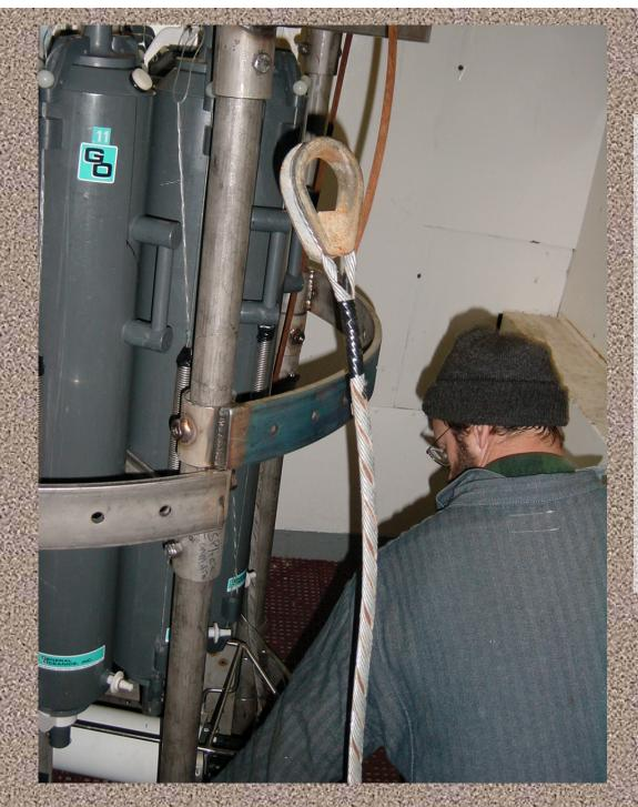
To increase termination strength, a 1/2" Crosby cable clamp can be used to secure the eye end of the grip. To prepare for this, wrap several layers of electrical tape at the base of the eye. This provides a base for the cable clamp to grab.
