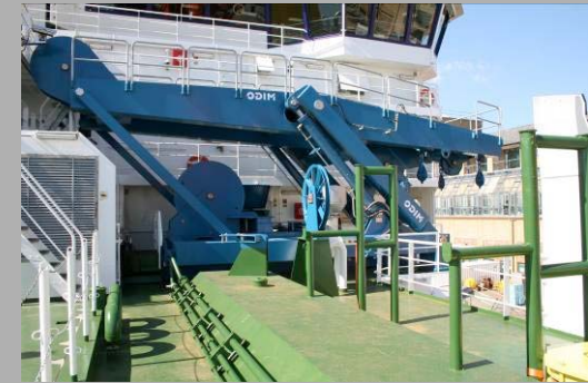
Starboard 'A' Frame Capacity – 30t Max. Height – 5m
