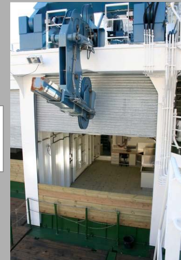
Starboard Hydro boom Capacity – 5T Max. Height – 4.5m
