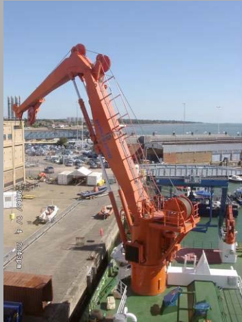
Midship/aft Crane 250 tonnes.m
