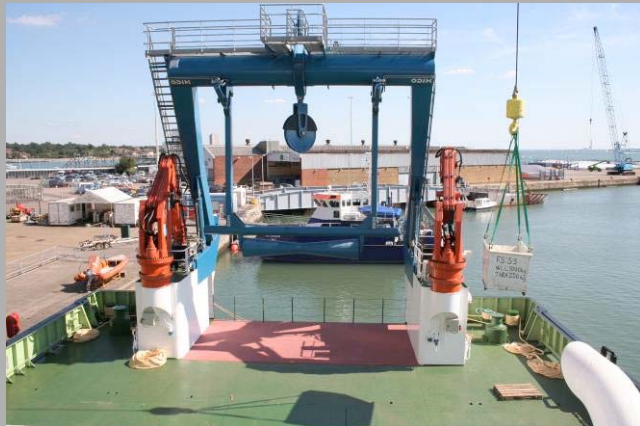
Stern 'A' Frame Capacity – 30t Max. Height – 8m
