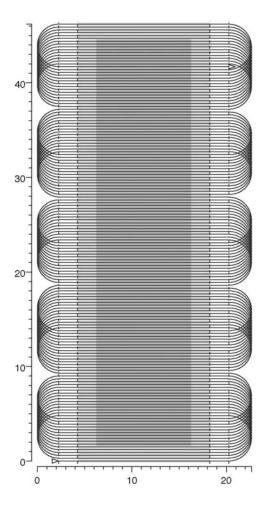
4 6000 m. streamers, 150 m separation 25 loops, 3 racetracks
