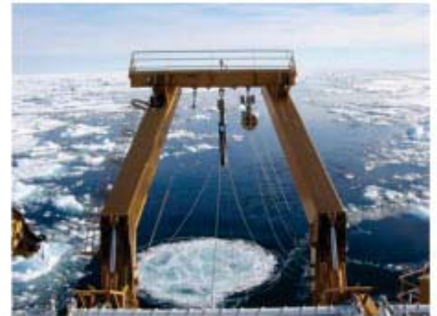
Figure 4. View of seismic source frame from above. Frame towed by main trawl wire.
