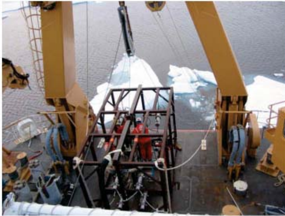
Figure 4. View of seismic source frame from above. Frame towed by main trawl wire.
