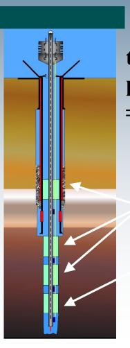
thermistors, pressure sensors, ± seismometer *CORKS*
