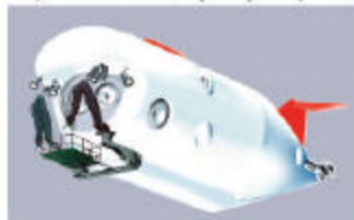
Conceptual drawing of the deep-diving human occupied vehicle under design as a replacement HOV. Illustration by E. Paul Oberlander, Woods Hole Oceanographic Institution.
