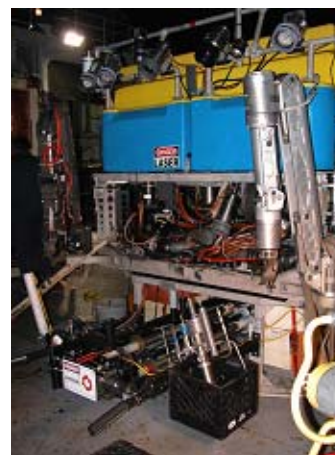
Jason2 with rock drill. Photo by Mitch Elend (UW) and Deb Kelley (UW)
