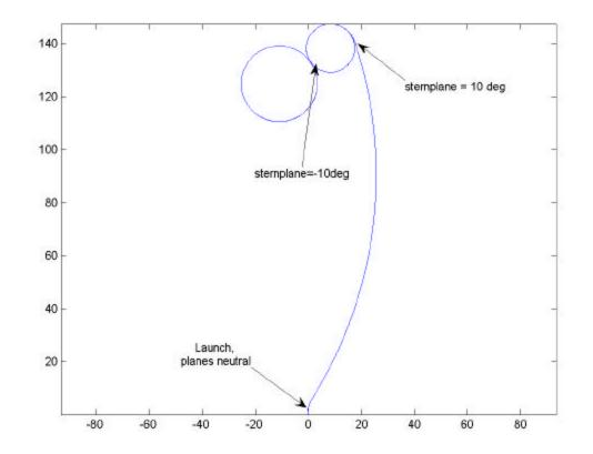
This plot shows the horizontal vehicle track for two sternplane deflections and offset descent weight.
