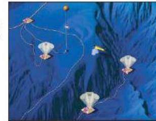
One element of the ocean observatories actively being planned for is a cabled network of linked sensors and submersibles spread out over the sea floor.
