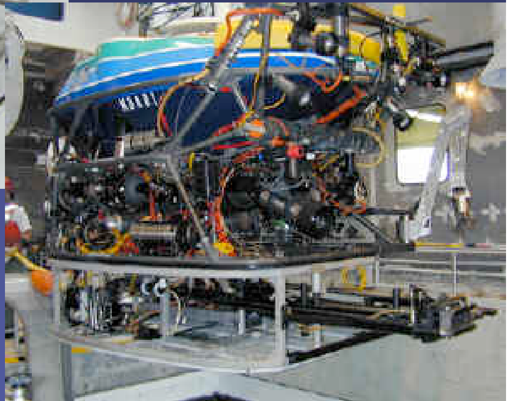
Drill sled mounted beneath Tiburon ROV
