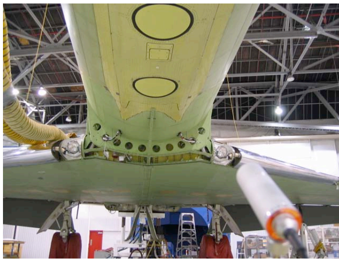
HIAPER undergoing High Blow Test (17.5 PSI) Note nadir ports with plate covers.
