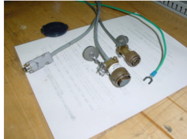
Deck Cable – Lab End RS422 from Tow body
