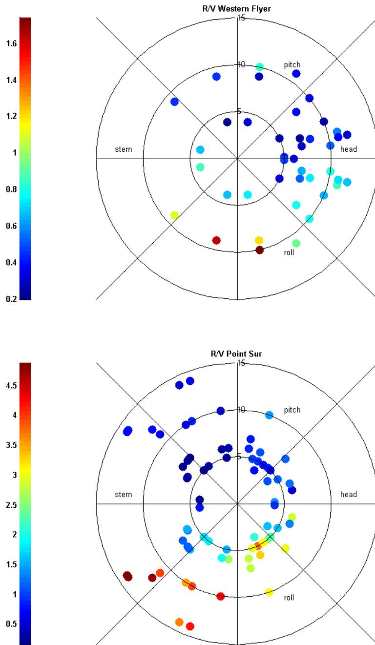
Figure 11. RMS pitch and roll at cruising speed. Data points are plotted at the head of a vector. The magnitude of the vector is the combined wave and swell height which is zero at the origin and increases to 15 feet at the outer circle. The direction of the seas wave are relative to the ship's head to the right and symmetric response was assumed. Pitch results are shown in the upper hemisphere and roll in the lower hemisphere. (upper) *Western Flyer*. (lower) *Point Sur*.
