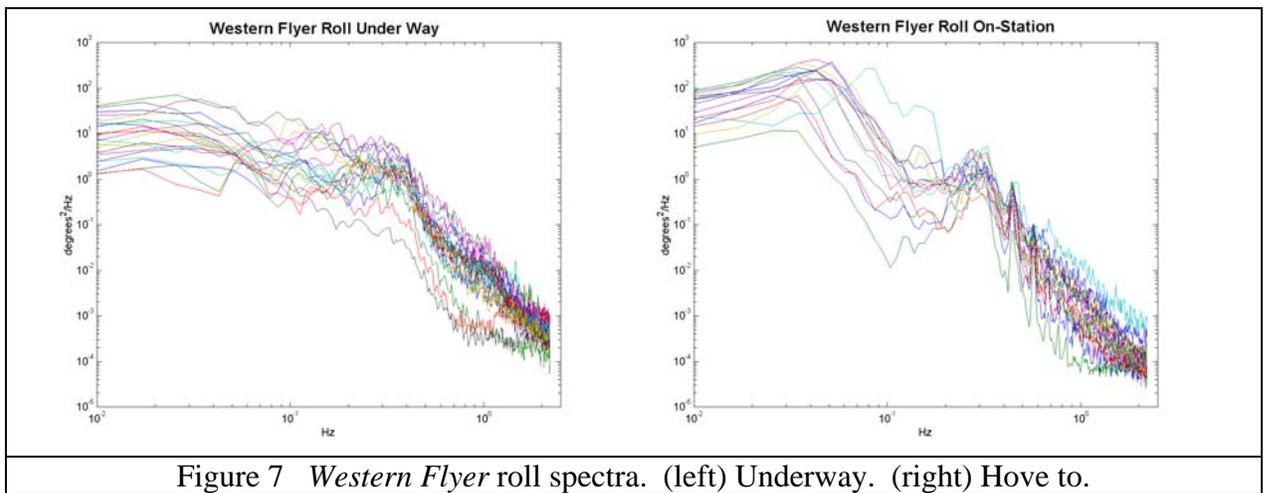
Figure 7 *Western Flyer* roll spectra. (left) Underway. (right) Hove to.
