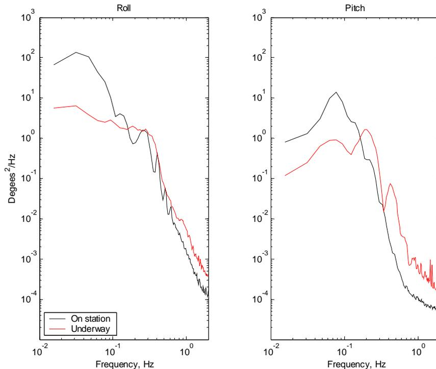
Figure 9. Mean spectra for the May 2003 *Western Flyer* cruise. The underway spectrum is shown in red and the on station spectrum is black. (left) Roll. (right) Pitch.
