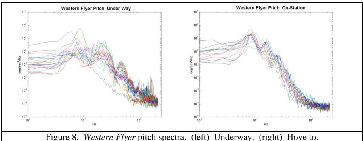
Figure 8. *Western Flyer* pitch spectra. (left) Underway. (right) Hove to.
