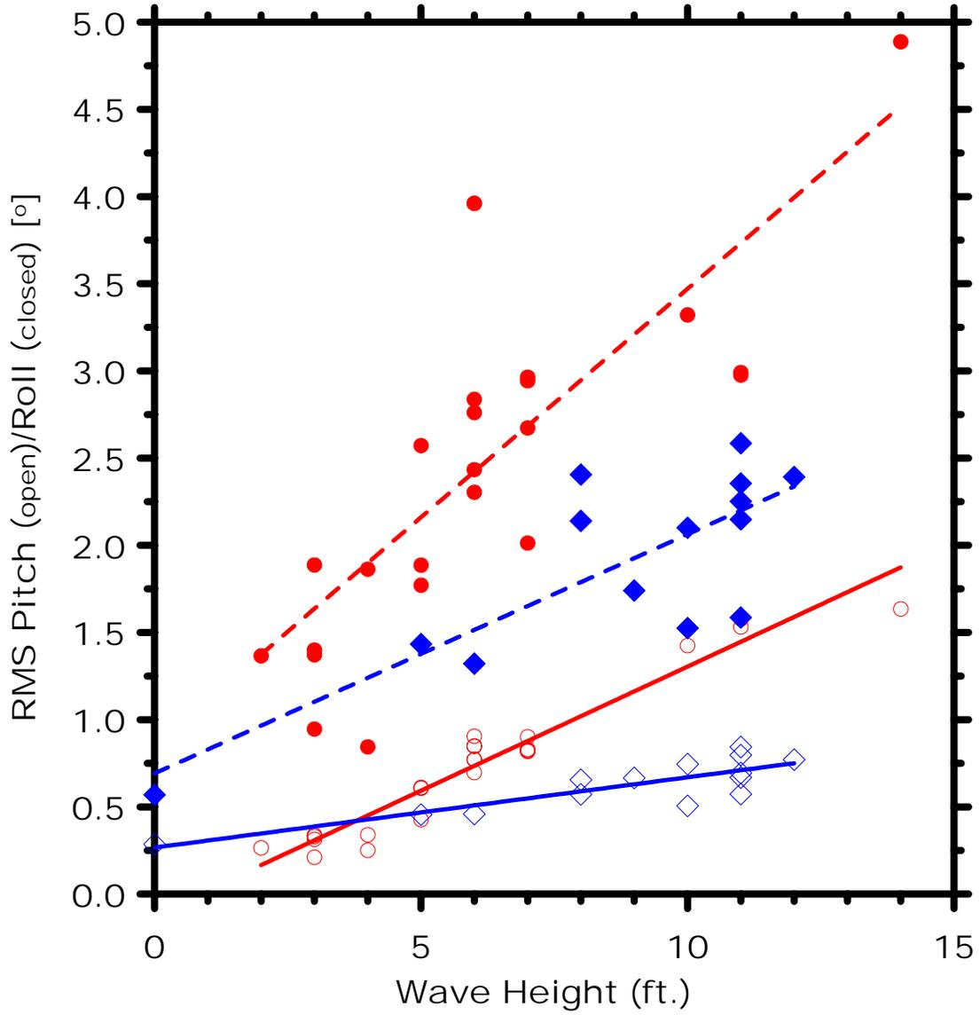
Figure 10. RMS pitch (open symbols) and roll (closed symbols) as a function of combined wave and swell height while vessels were hove to with their head into the seas. *Point Sur* data are shown in red and *Western Flyer* data are in blue. Lines were fitted to data using the method of least squares.
