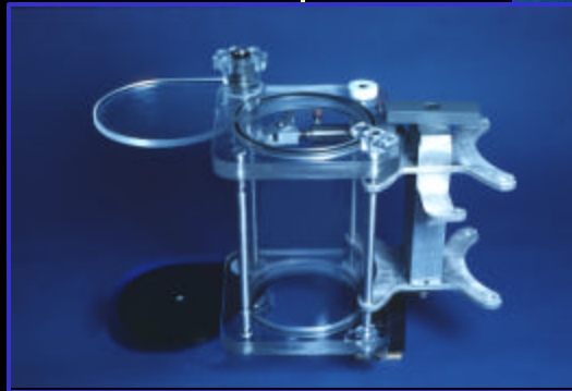
SAMPLER FOR GELATINOUS ZOOPLANKTON
