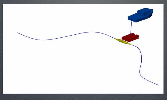
FAILURE IN NODE BRANCHING UNIT REQUIRES LIFTING NBU PLUS TWO ATTACHED CABLES
