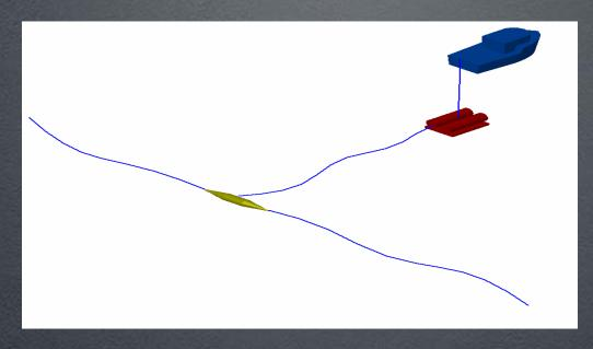
J-BOX IS HARDWIRED TO SPUR CABLE FROM BACKBONE
