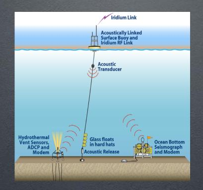
Single point, semi-taut surface mooring with acoustic link Installation from large UNOLS vessel is routine No ROV required for installation or maintenance
