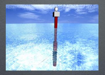
40 m long spar buoy with diesel generators and radome Three point mooring with electro-optical link to j-box Installation and instrument maintenance will require an ROV Installation and buoy maintenance not feasible with largest UNOLS vessels
