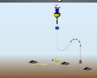
Single point mooring with electro-optical S-link 2.4 m discus buoy Installation from large UNOLS vessel is feasible ROV required for installation and maintenance
