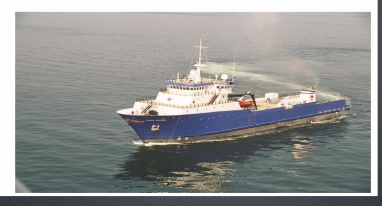
MULTI-PURPOSE HEAVY LIFT VESSEL OPERATED BY OCEAN SERVICES LLC 273' LOA, 2700 GT , 3 HOLDS FOR CABLE/CARGO TWIN 1500 HP MAIN PROPULSION, 1000 HP TUNNEL AND AZIMUTHING BOW THRUSTERS, TWIN 1100 HP AZIMUTHING STERN THRUSTERS LARGE OPEN DECK SPACE AFT 65 TON CRANE
