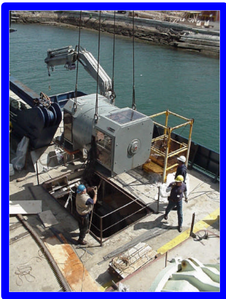
Removal of Port Motor on Atlantis
