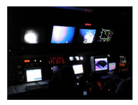
The Control Van is where Pilots, Navigators, and Engineers control remotely operated vehicles (ROV) such as Jason and Argo. Scientists use these vehicles for underwater scientific research.
