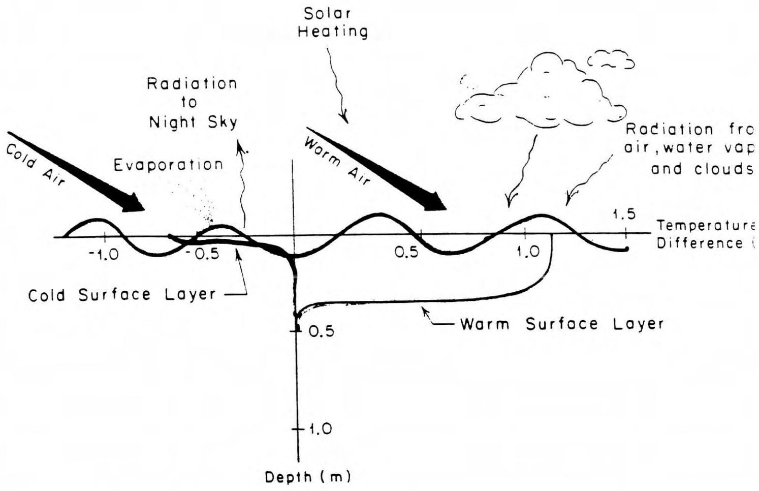
Figure 8.1 Processes influencing the temperature of the skin of the ocean. The skin temperature is measured by infrared radiometers, and it may not be representative of temperature slightly greater depths.
