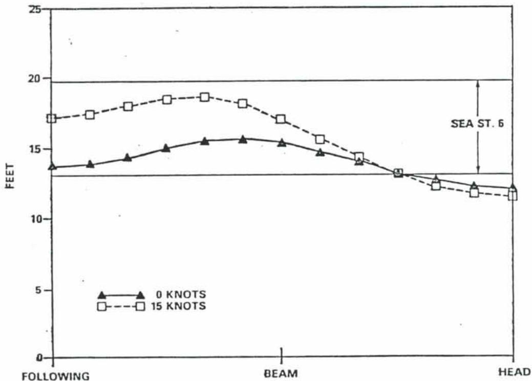
Figure 3.6. Limiting Significant Wave Height - New Construction Monohull Baseline
