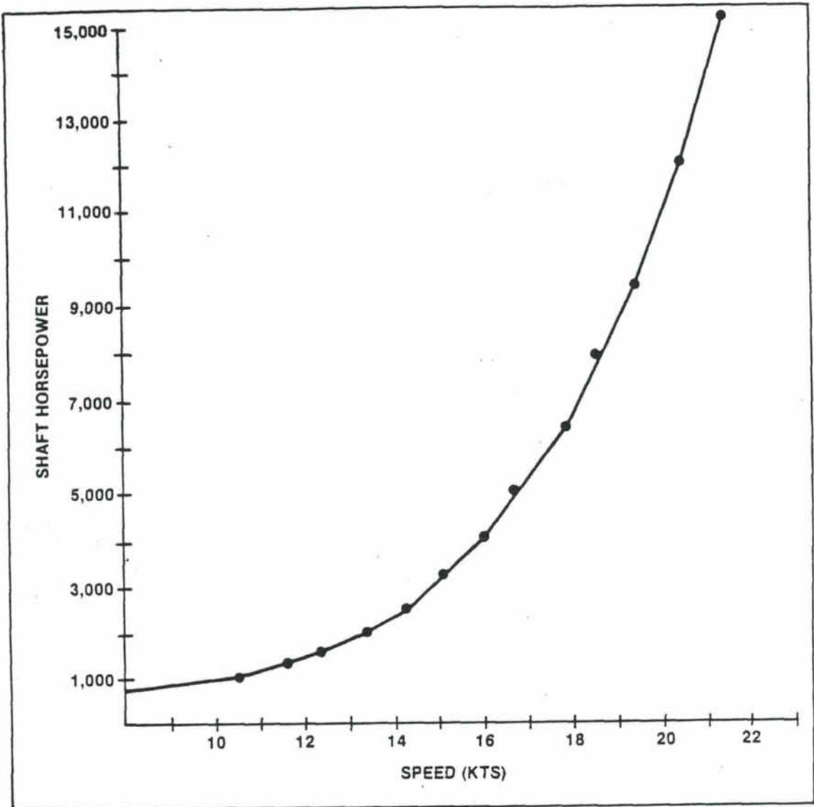
Figure 3.3. Speed/Power Curve for AG(X) Monohull
