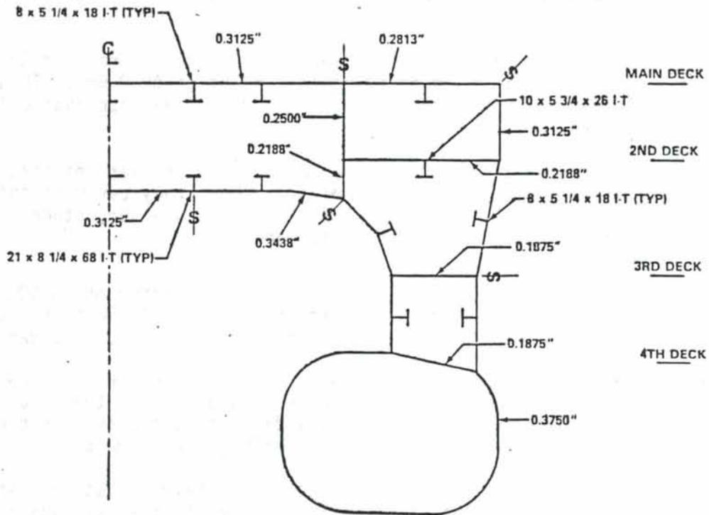
Figure 4.2. Midship Section of SWATH Structure
