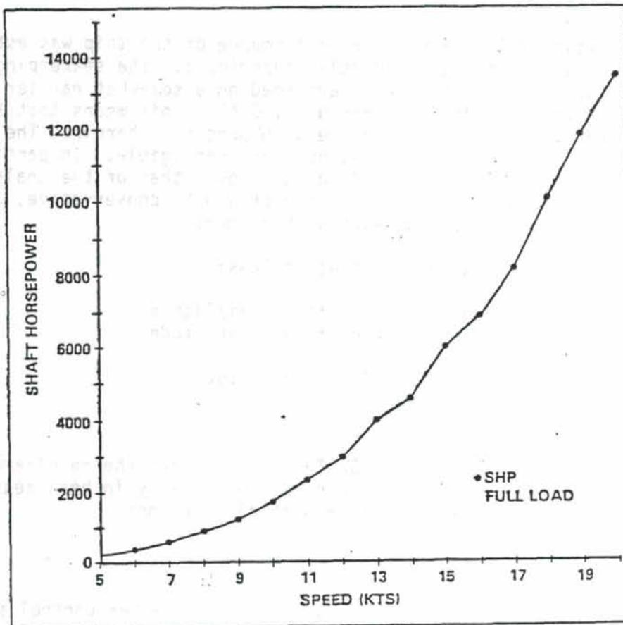
Figure 4.3. Speed/Power Curve AG(X) SWATH
