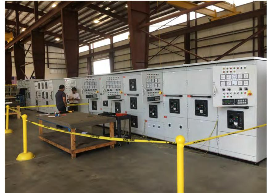
New switchboards undergoing Factory Testing
