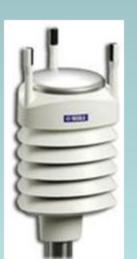
Pressure sensors are similar with varying response times and accuracies depending on your need. For shipboard use it is critical to have a dynamic pressure port connected to the sensor to reduce the dynamic wind effects (Bernoulli Effect). This pressure port should be located in a place on the ship least affected by flow around the ship's structure. Note: The actual pressure is measured at the height of the sensor and not the pressure port. The plot is a comparison of 2 different
