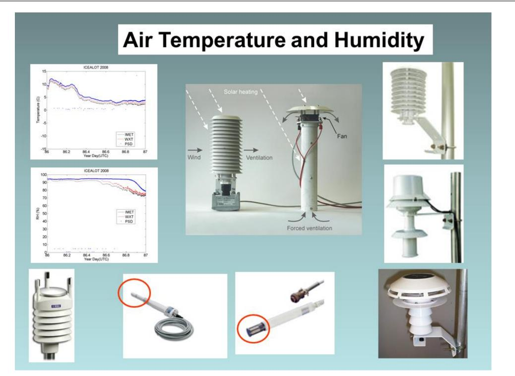
Plots are comparisons between three different sensors. Red circles indicate where actual T/RH sensors are located. These fit up into a radiation shield shown on the right side. Radiation shields can either be naturally ventilated (top) or fan driven (bottom two).
