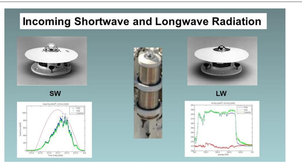
SW (Pyranometer) broadband solar radiance on a planar surface LW (Pyrgeometer) atmospheric infra-red radiation. Good quality radiometers are not cheap but very important to understanding the energy budget. Plots show comparisons between ship (SCS) and Flux Standard (PSD) sensors along with modeled clear sky calculation for incoming SW and downwelling LW radiation.
