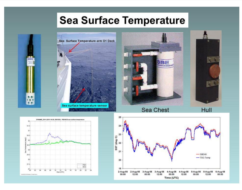
Sensors from left to right: temperature profiling sensor typically used with CTD, "Seasnake" floating thermistor, ship intake, hull mounted. Left plot shows comparison between "Seasnake" (blue) and ship intake sensor (green) with warming caused by heating from the sun of the "Seasnake". Right plot is comparison of ship intake (blue) and hull (red) sensors showing dampening and delay of hull mounted temperature sensor.
