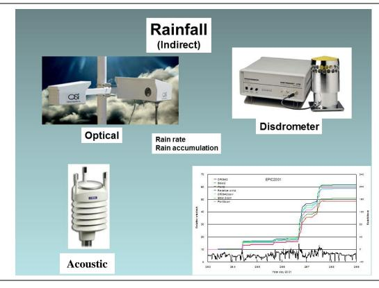
Indirect methods for measuring precipitation. Optical (most common for ships). Plot shows comparisons for different sensors and different locations with ship relative wind speed plotted along the bottom. All sensors capture the various rain events,
