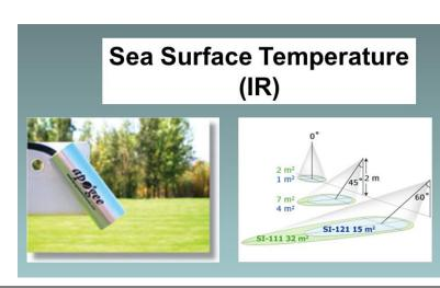
Indirect measurement using IR sensor. Total surface area viewed dependent on tilt angle of sensor.
