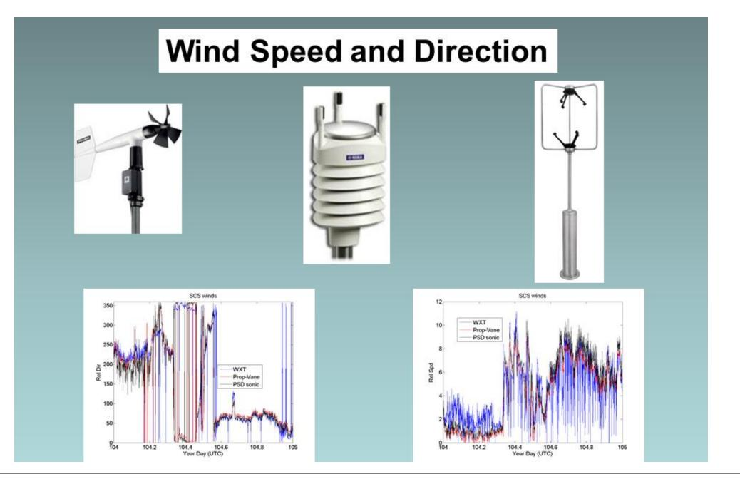
**Prop-vane anemometer, 2-D sonic anemometer, 3-D sonic anemometer** The two main methods of measuring winds are either mechanical or indirect via sound. They are often both obtained from a single instrument and are measured relative to the ship and therefore must be combined with the ship's heading, course, and speed to arrive at the true wind vector. Plots show comparisons of True wind direction and speed from the three different wind sensors pictured
