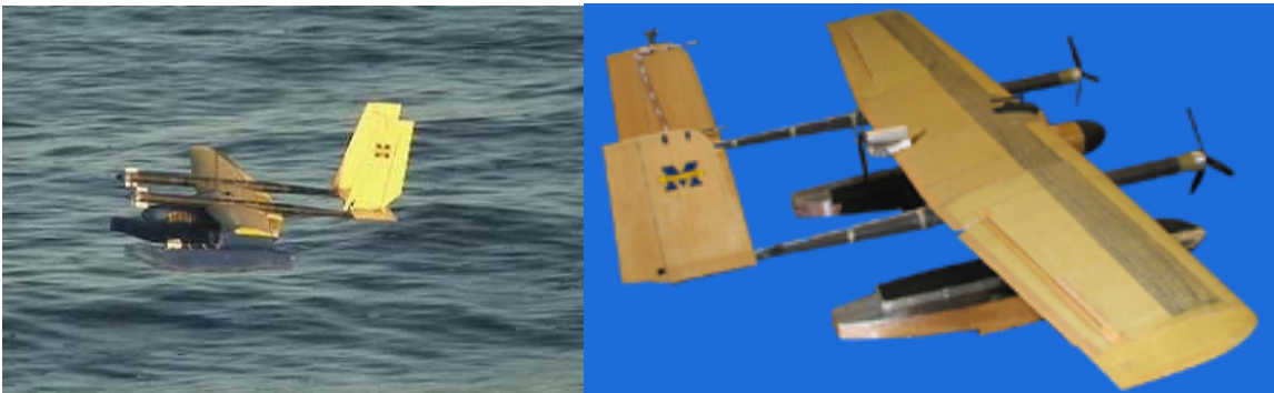
Figure 11. The Searobotics Unmanned Survey Vessel (left) is intended for riverine and coastal surveys, while the Self-Righting Monohull (right) is intended for multibeam surveys in rougher waters.
