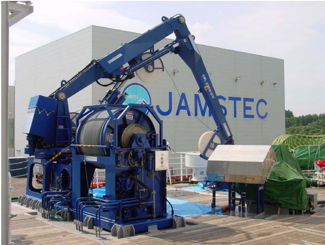
Figure 21. Nodding boom with tension adjusting winch shown on Japanese research vessel.
