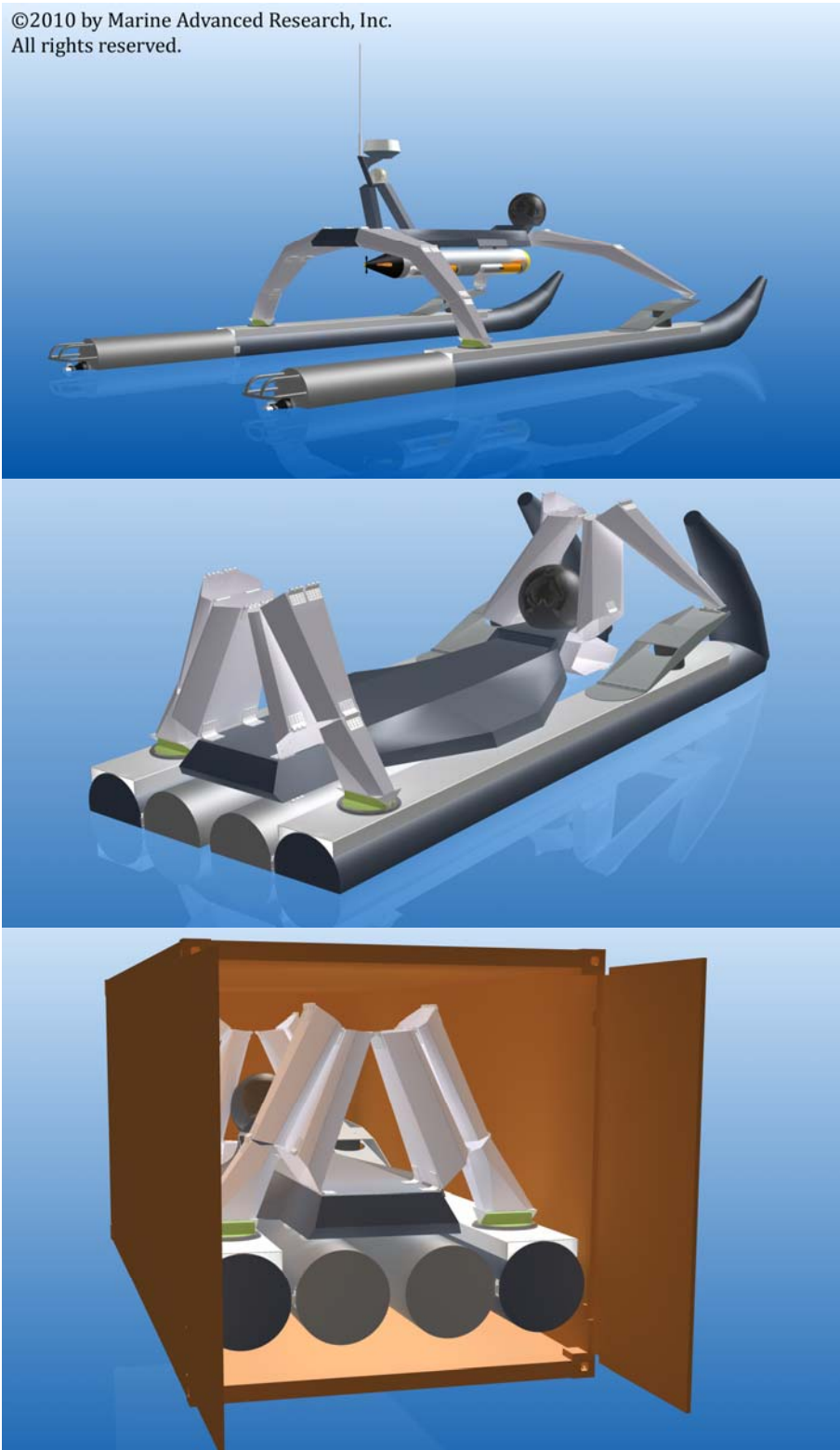
Figure 15. Sketches of 33' WAM-V (Wave Adaptive Modular Vessel) carrying UUV for deployment (top), folded for launch and retrieval (center), and folded for shipping into a 20' shipping container (bottom).
