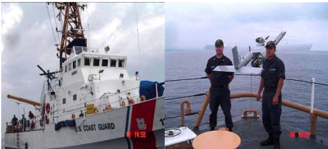
Figure 6. Shipboard launch system for Silver Fox on a Coast Guard 110' Coastal Patrol Boat off Hawaii in 2006 mounted on upper deck.
