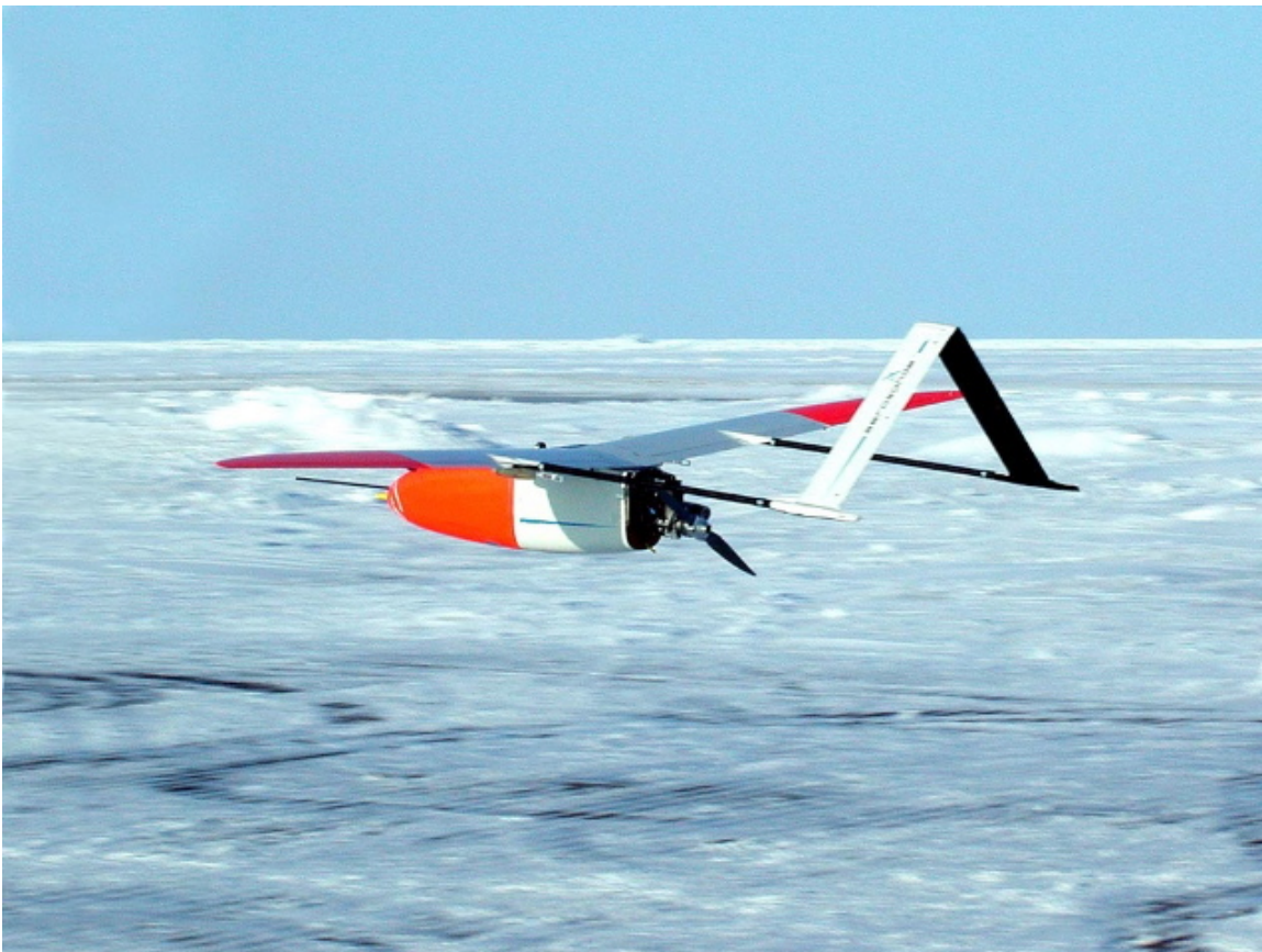
Figure 8. The Aerosonde UAS has been used for high latitude reconnaissance missions including studies of sea ice and glaciers, but to date has been launched only from land, with recovery on ice or sandy beaches. The broad array of sensor packets developed for it may soon see it used from ships at high latitudes including icebreakers, while continuing to rely on sea ice or beach landing and recoveries.
