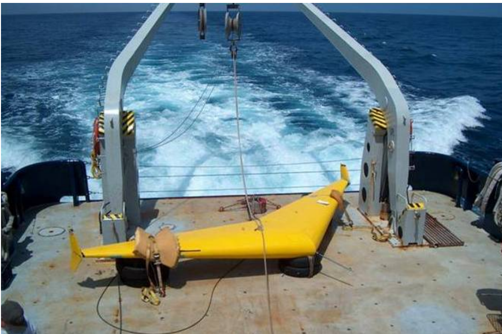
Figure 20. The Scripps Flying Wing style UUV, built for the Navy, requires not only considerable deck space for storage, but also care in launching and small boat retrieval and recovery.
