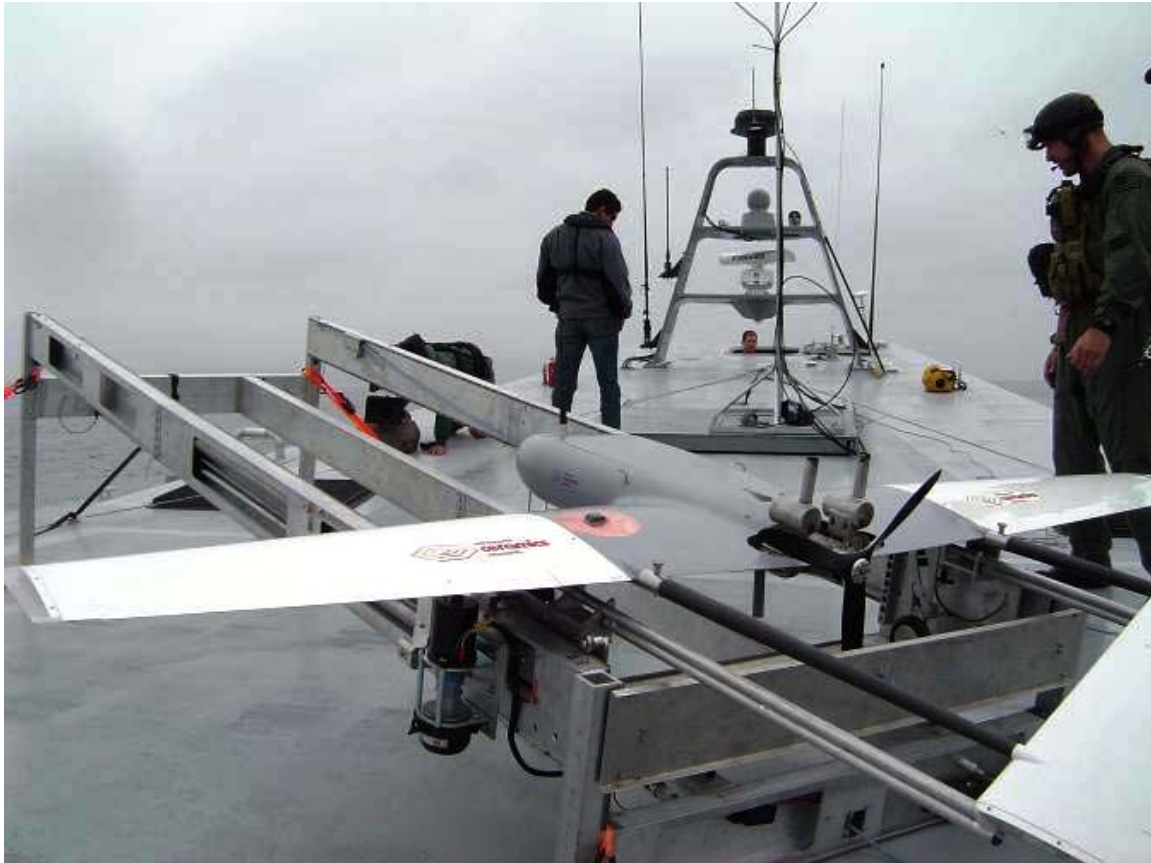
Figure 6. Shipboard launch system for Silver Fox on a Coast Guard 110' Coastal Patrol Boat off Hawaii in 2006 mounted on upper deck.
