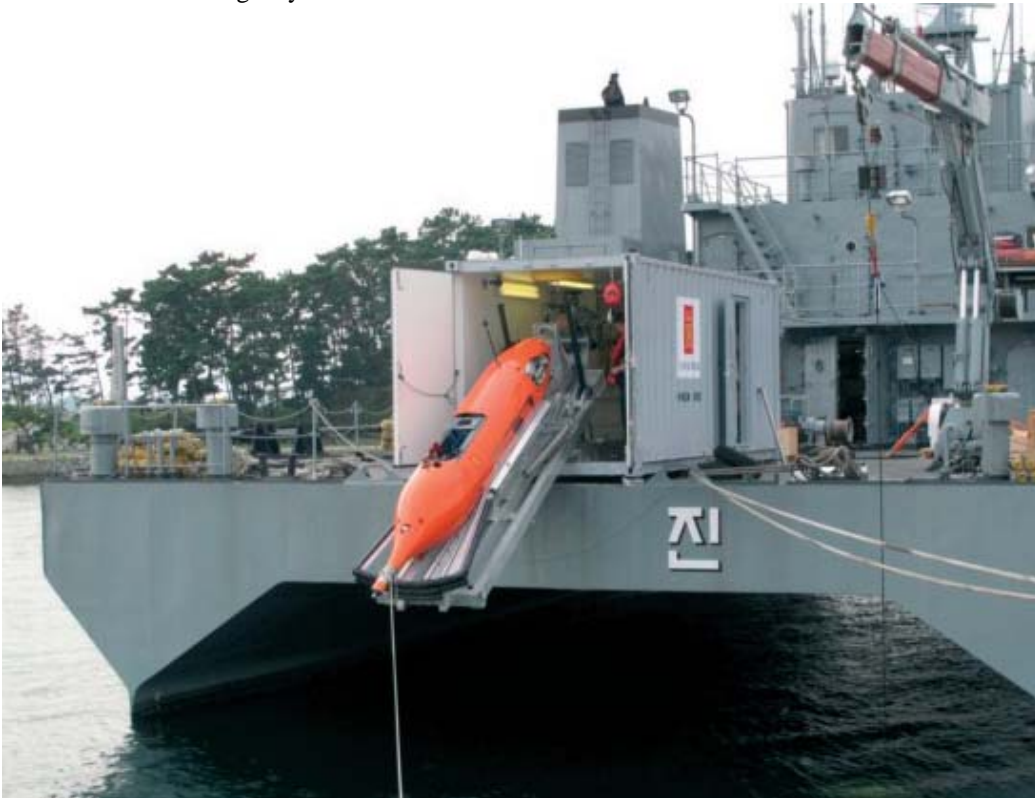
Figure 20. The Scripps Flying Wing style UUV, built for the Navy, requires not only considerable deck space for storage, but also care in launching and small boat retrieval and recovery.
