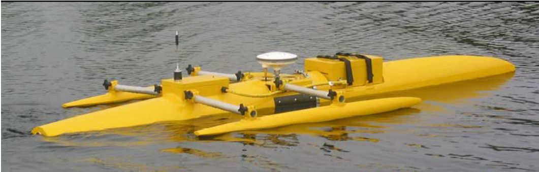
Figure 13. The Wave Glider Unmanned Surface Vessel manufactured by Liquid Robotics is now becoming widely used by the Navy is designed to be deployed and recovered by two individuals or through use of a small shipboard crane or small boat. Versions with marine meteorological sensors (top) and surveillance camera systems (below) are among several that have been developed.
