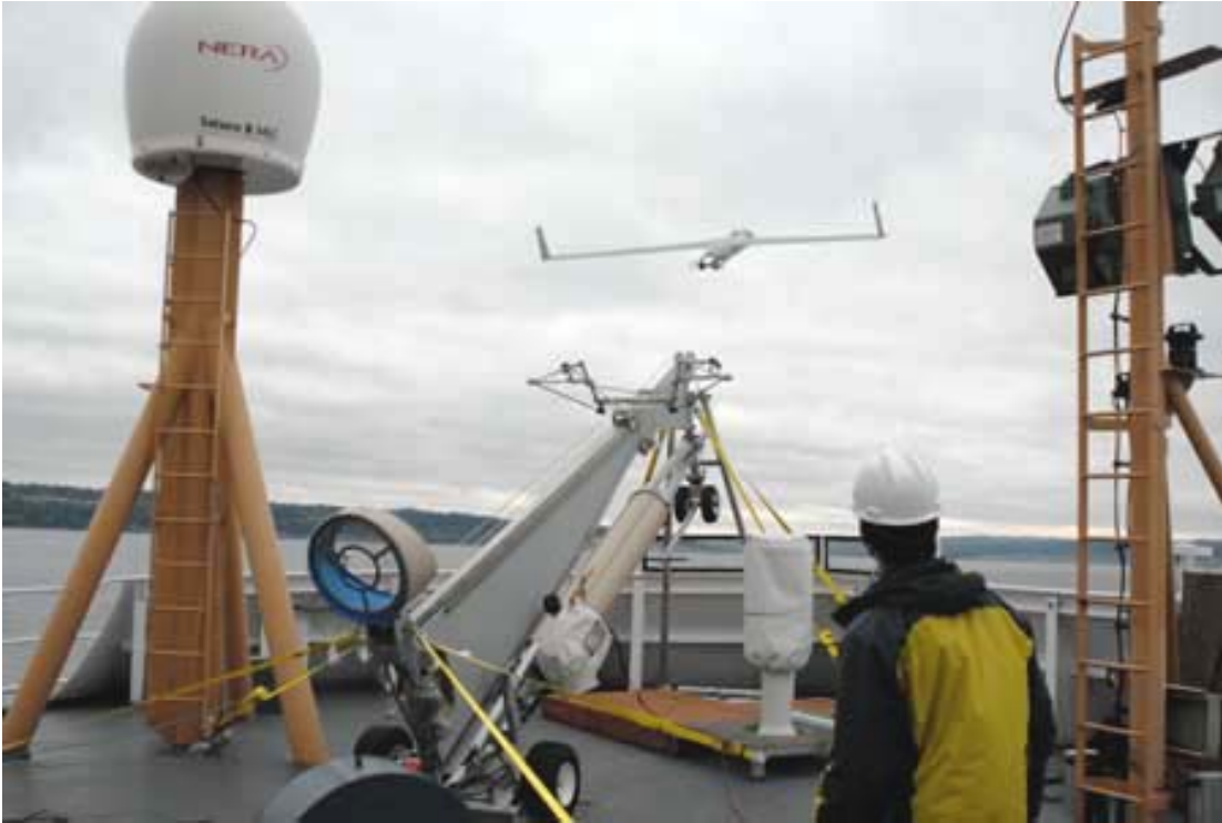
Figure 2. Recovery of ScanEagle Unmanned Aircraft in 2009 from NOAA Ship McARTHUR II.
