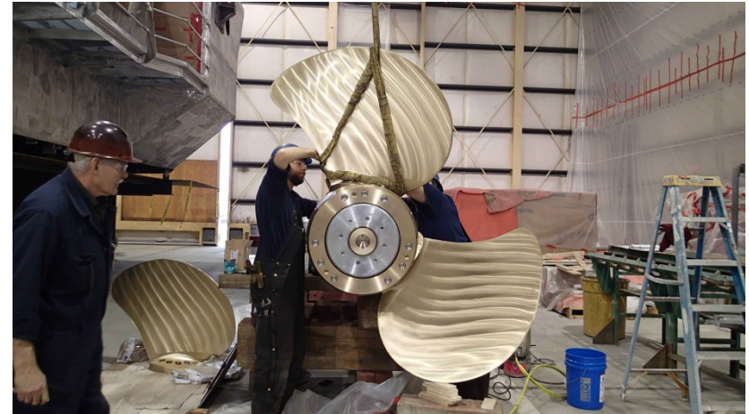
Controllable Pitch Props being assembled
