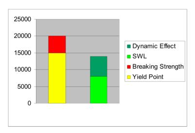
A.4.7 When a tension measuring system is not available which forces using a minimal FS of 5.0, estimates of tension due to "dynamic loading" must be done based on mass not weight. In general, the weight of the package, entrained water and the cable or rope in air is roughly equal to the mass. Do not use weight in water for the dynamic loading estimates.
