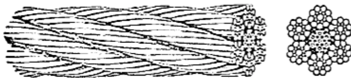
6 x 19 Searl Right Regular Lay, IWRC
