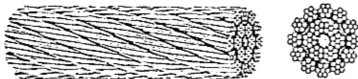
18 x 7 Non Rotating, Fiber Core
