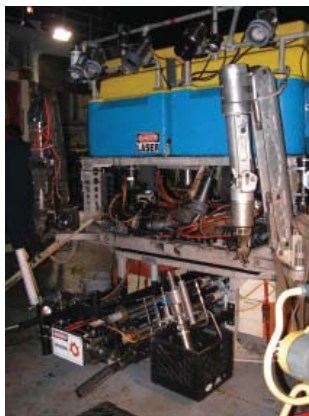
ROV Jason2 with Rock Drill. Photo by: Mitch Elend (UW) & Deb Kelley (UW)
