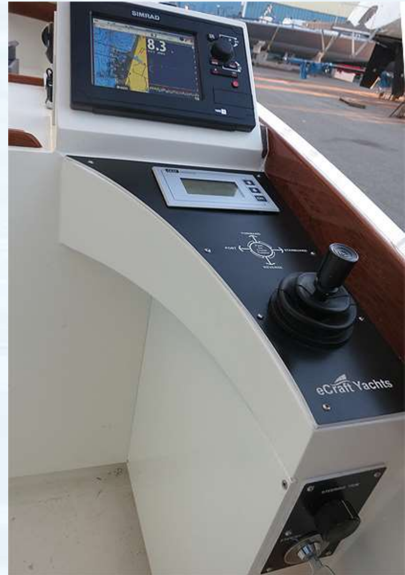
Joystick for throttle and steering
