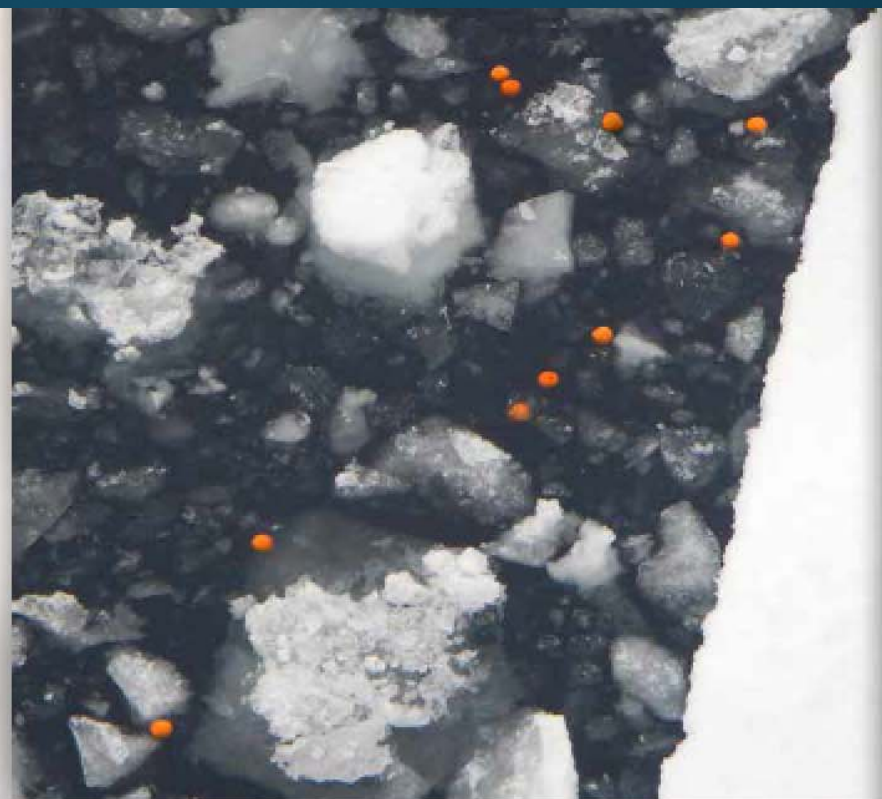
Oranges thrown in ice-infested Arctic waters to simulate an oil spill. Photo credit: USCG
