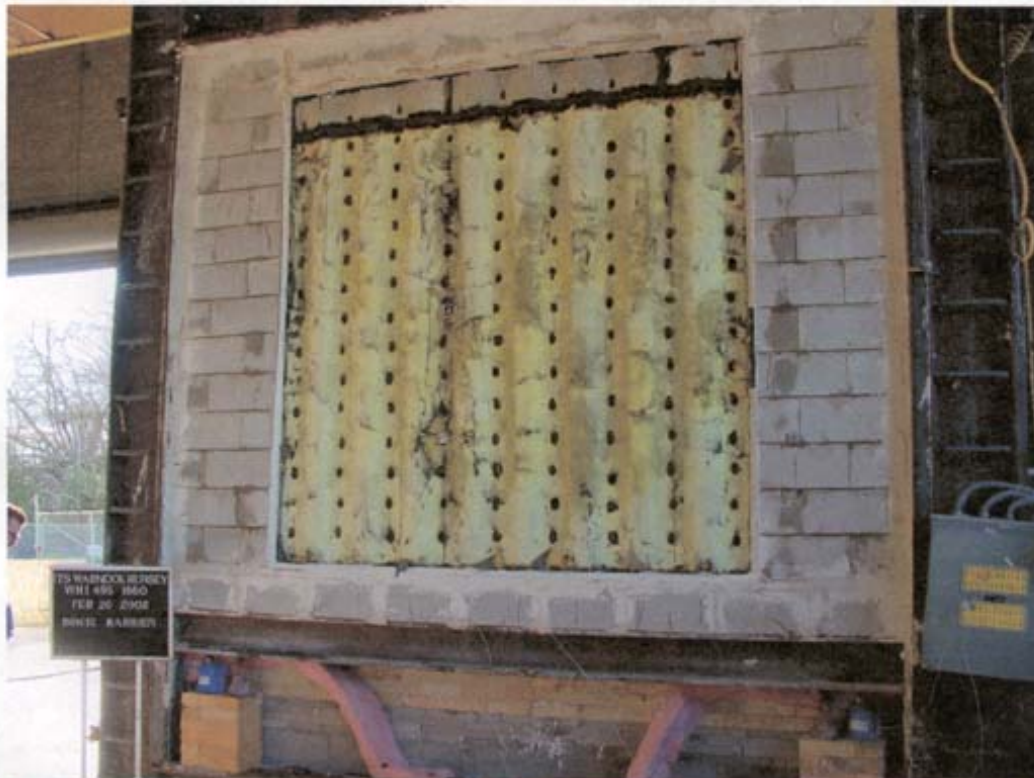
Test WHI-495-1660: After Fire Endurance Test
