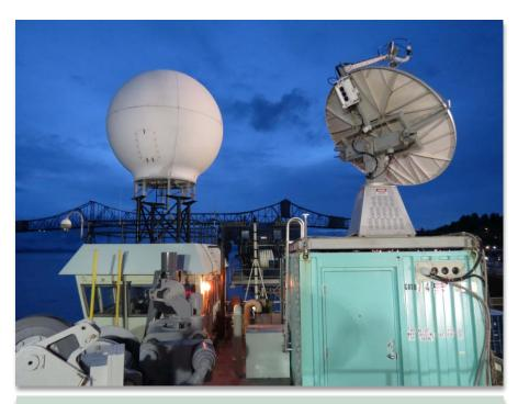
FIG. 5: RESEARCH SHIPS ARE SUPPORTING INCREASING LEVELS OF TELEPRESENCE ENABLED BY SHIPBOARD NETWORKS, NEW SENSORS AND SATELLITE COMMUNICATIONS. THE VAN IN THIS PHOTO CONTAINS A MOBILE TELEPRESENCE SYSTEM INSTALLED ON THE **R/V** *Atlantis*.
