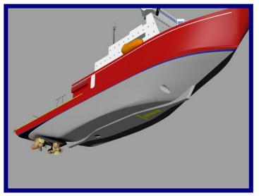
Fig. 2: Underwater view of PRV box keel with bottom mapping sensors
