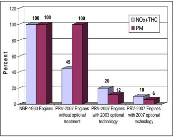
Fig. 4: Emission reduction per horsepower
