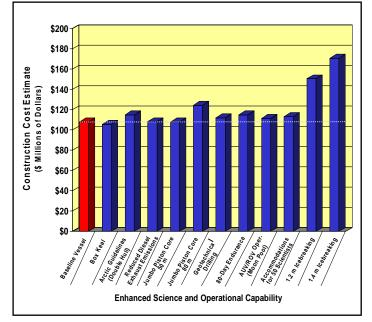
Fig. 7: Significance of individual mission requirements on construction cost
