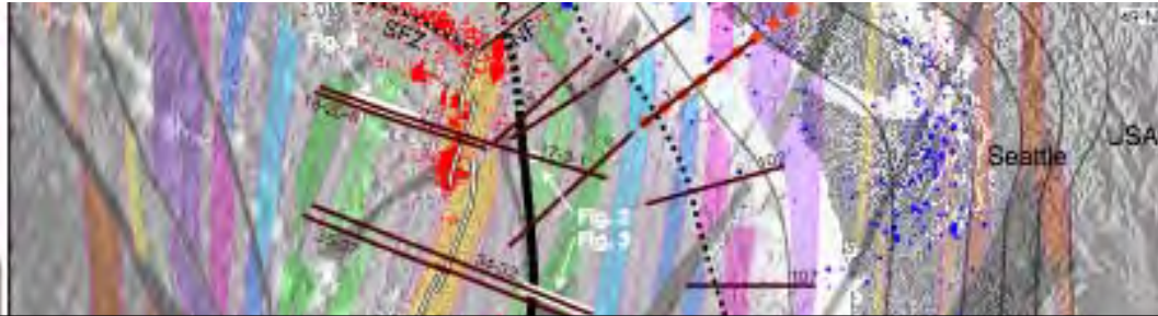
2012 RV Langseth 40 guns, 6,600 c.i., 2000 psi, 37.5 m. 636 channels. Fold: 105
