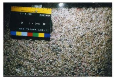
Figure 081-1-1 (SH10) FR-50, Over 100 Percent Of Area (Sheet 10 of 22). Source: S9086-CQ-STM-010, Chapter 081, Waterborne Underwater Hull Cleaning of Navy Ships
