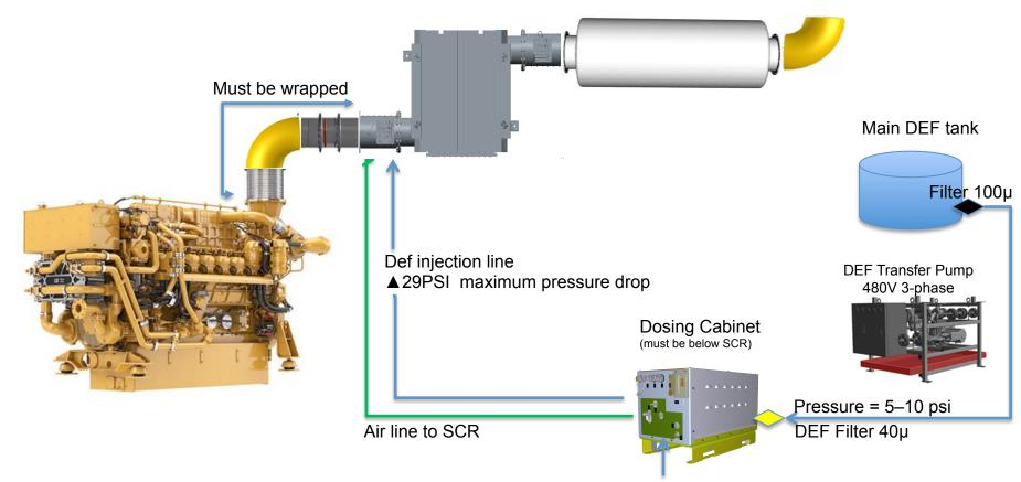
Air flow = 10CFM (4CFM for C32) Air pressure = 80-150 psi ( See A&I guide)
