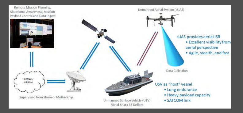
Optionally Manned Metal Shark Defiant 38 Patrol Boat with VTOL UAS and Over the Horizon Communications (11.5m / 40+ knots)
