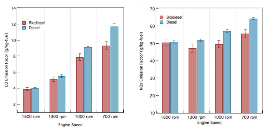
Emission factors of CO and NOx from R/V *Robert Gordon Sproul* at different engine speeds when powered by diesel and biodiesel. Each mean represents the average of a number of one-hour test periods (n=7 for biodiesel; n=2 for diesel). The average was calculated over different engine cycle tests conducted during a 2015 cruise.
