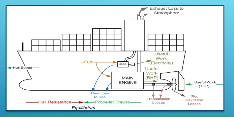
Minimize losses in conversion of chemical fuel energy to rotational torque energy from engine
