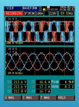
Voltage and Current wave form with VFD
