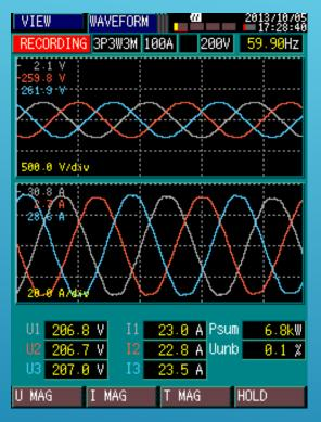
Voltage and Current wave form without VFD VFD: Introduce harmonics into the motor
