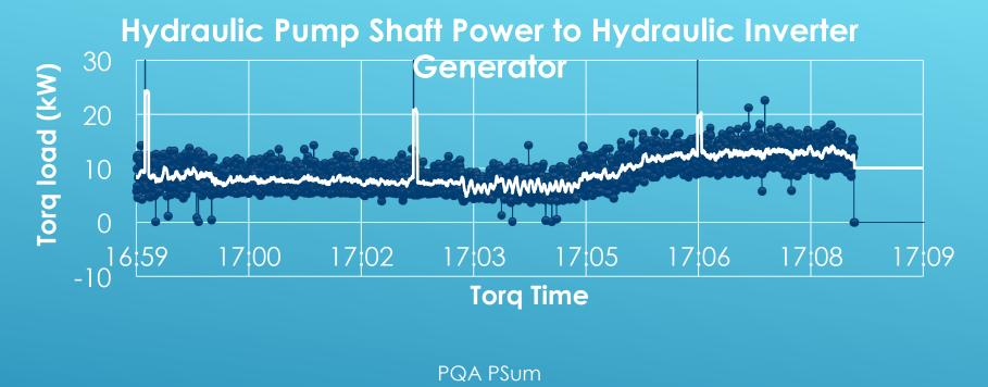
Losses in converting shaft power to hydraulic power to electrical power
