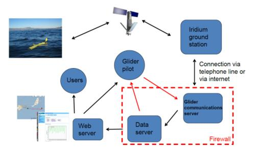
Figure 4.2 shows the operational connectivity used by Principal Scientists to fly gliders in support of their MSR RO.
